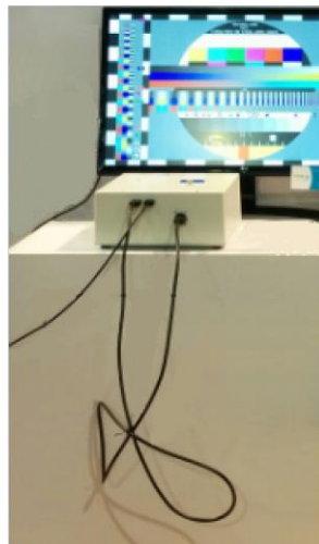
Figure 2.9. CISPR recommended DUT cable placement inside chamber
