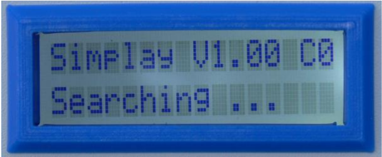
Figure 2.4. SL-889 Operation: C0 Resolution, V1.00 Firmware, No HDMI Cable Attached
