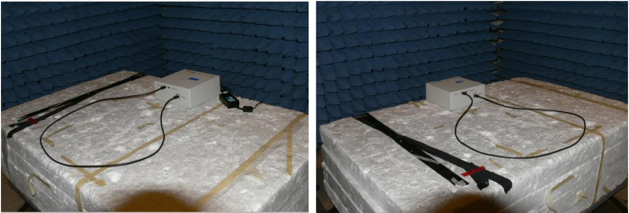
Figure 3.3. HDMI Forum recommended DUT cable placement inside chamber
