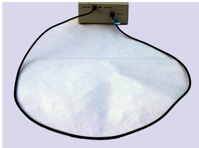
Figure 2.10. HDMI Forum recommended DUT cable placement inside chamber
