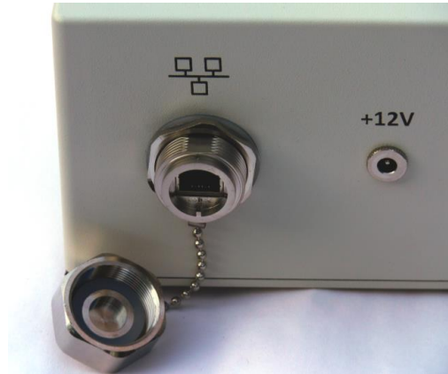
Figure A.3. SL-889 Firmware update via network port
