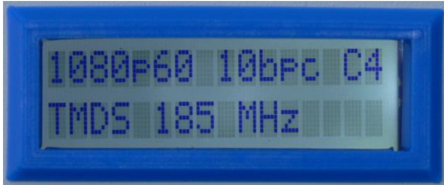
Figure 2.7. SL-889 Operation: C4 Resolution, TMDS 185 MHz link, HDMI Cable Attached
